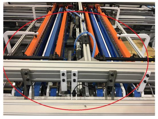
THERE ARE SIX BRIDGES ,SIX THIS KIND MOTORS AND SIX BTTONS . EACH BUTTON ADJUST ONE BRIDGE BY ONE SERVO MOTOR .
