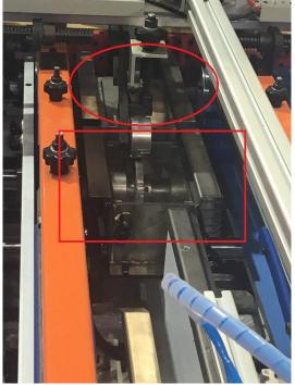
TWO GLUE TANKS IN THE MIDDLE , ONE IS HOT GLUE AND ONE IS COLD GLUE .
