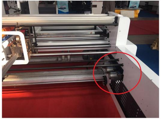
EACH BRIDGE CONTROLLED BY EACH SERVO MOTOR ( WHICH MAKRED BY CRICLE ).
