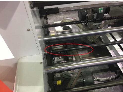
THE KNOB CAN ADJUST THE TWO GLUE TANKS IN THE MIDDLE , LEFT AND RIGHT . NO NEED TO GO ON TOP OF THE MACHINE AND NO NEED TO LOOSE ANY SCREW . IT IS MORE CONVENIENT AND SAVE A LOT TIME .
