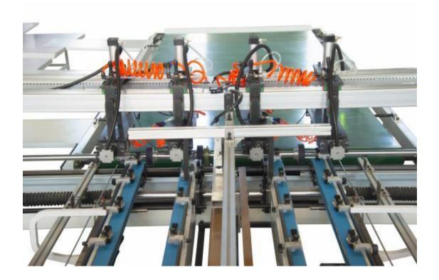
The paper feeding section of the main machine adopts four paper belt wall plates that can be adjusted to move;
