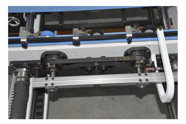
Side pushing paper positioning department on both sides of the patting paper using two sets of servo system drive four sets of precision ball screw side pushing positioning,
