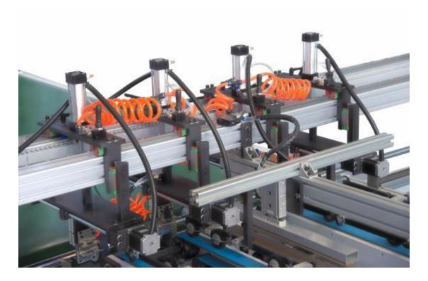
The front gauge flush section adopts PLC-controlled servo system for precise digital positioning of the front gauge position, and the man-machine interface can store orders and adjust them digitally with one key,
