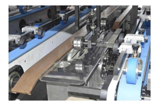
The gluing department adopts hot melt glue + sealing glue double coating method,
