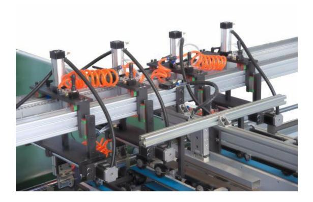
The front gauge flush section adopts PLC-controlled servo system for precise digital positioning of the front gauge position, and the man-machine interface can store orders and adjust them digitally with one key,
